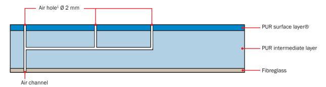
$<sup>^{\</sup>rm 1}$  Air hole arrangement only shown schematically. Design depends on adapter width and diameter.
